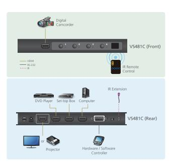
Note: Three HDMI In Ports are located on the rear panel, and one on the front.
